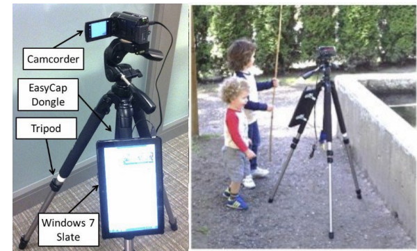
Figure 2: The Experiences2Go prototype combined a camcorder with a tablet used to show the remote person. E2G is shown at a family birthday party at a fish hatchery.
